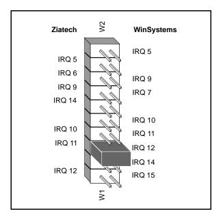
Figure 2-5 shows the setting for IRQ11 in a Ziatech AT-compatible computer.
